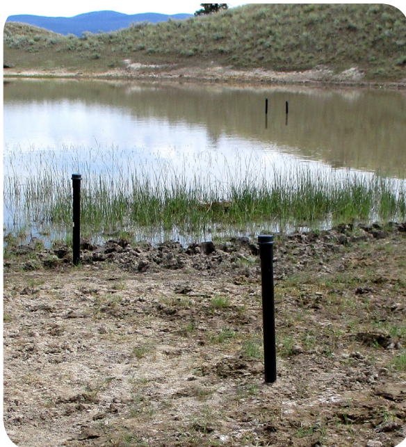
Data logger casings of a well to monitor water depth and 3 piezometers to measure ground water head in the wetland and adjacent riparian zone..
